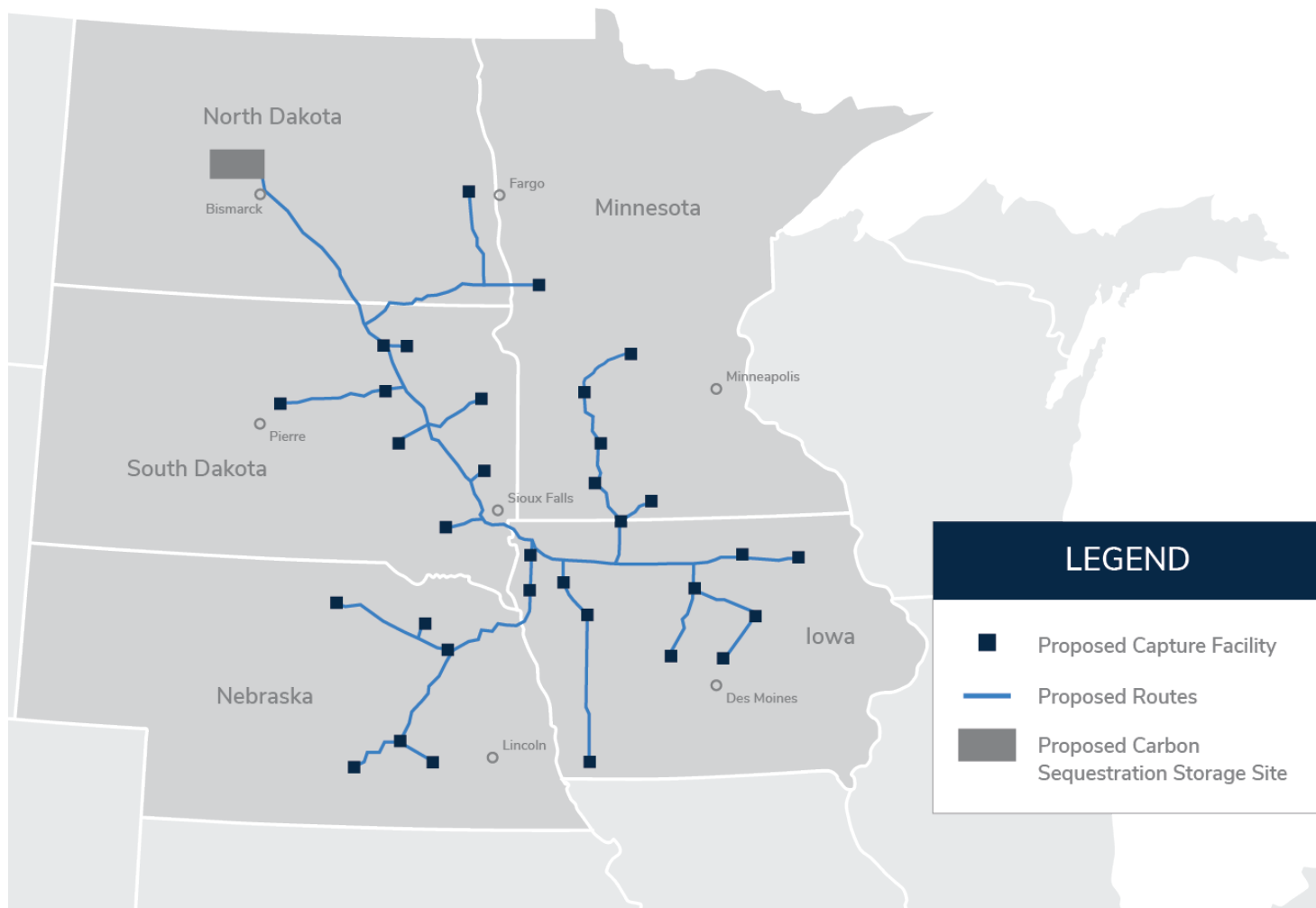
Summit Carbon Solutions has partnered with 30 ethanol plants to construct a project that runs across a five-state region
